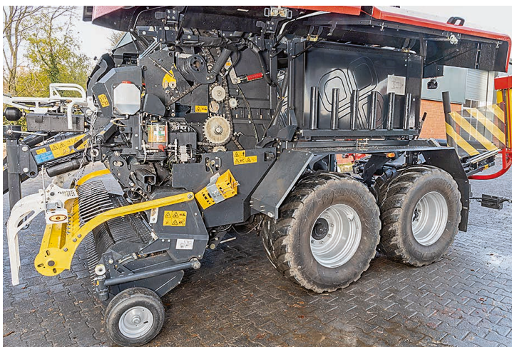
On the left are the oil and grease applicators as well as the chain driveline. The hydraulic components live on the right-hand side of the machine.
