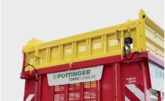
A sensor at the lower end of the front panel measures the loading pressure for damp, heavy grass and switches the scraper floor on and off accordingly.
