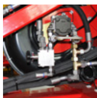
Load sensing fan drive system
