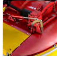
Hydraulic folding side guard
