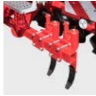
Spring loaded tractor track eradicators
