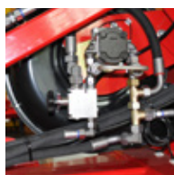
Load sensing fan drive system
