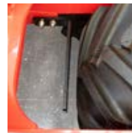
Scrapers for packer wheels
