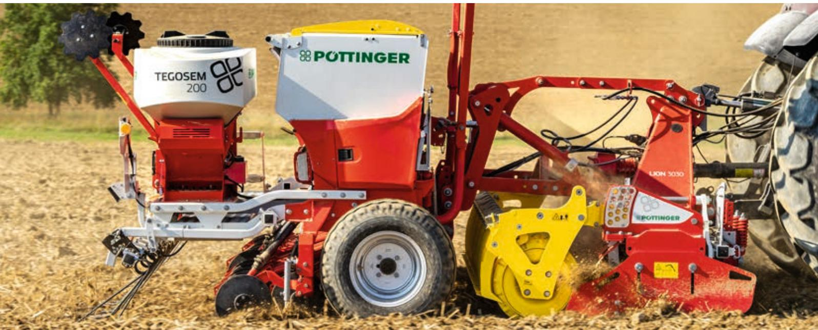
When the TEGOSEM is combined with seed drills and soil preparation implements, two processes can be carried out in a single pass. This is a fast and cost-effective way of sowing a cover crop or similar material at up to 40 kg/ha. As a result, it opens up a number of different capabilities with different machine combinations.
