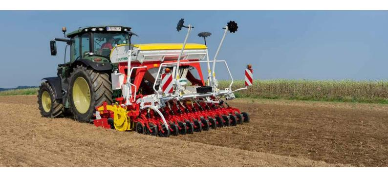
The unique AEROSEM seed drill concept unites the drilling of cereals and maize. Precision universal metering and coulter systems proven time and again in the field guarantee exact placement of the seed.
