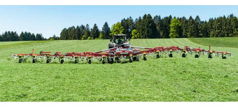
Our proven rotary tedders deliver perfect ground tracking. Both the mounted and trailed tedders feature jockey wheels located close to the tine arc to react to any bumps. In addition, all frame joints follow every contour independently of one another. The tines do not touch the ground. Tedding crops carefully without contamination entering the forage is the result.
