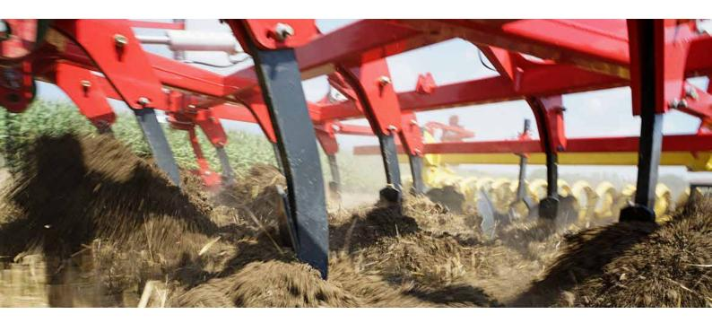
The PÖTTINGER SYNKRO stubble cultivators have been developed to deliver optimum stubble cultivation, and are suitable for both shallow and deep tillage. During the design phase, special value was placed on reducing draft and power requirements.
