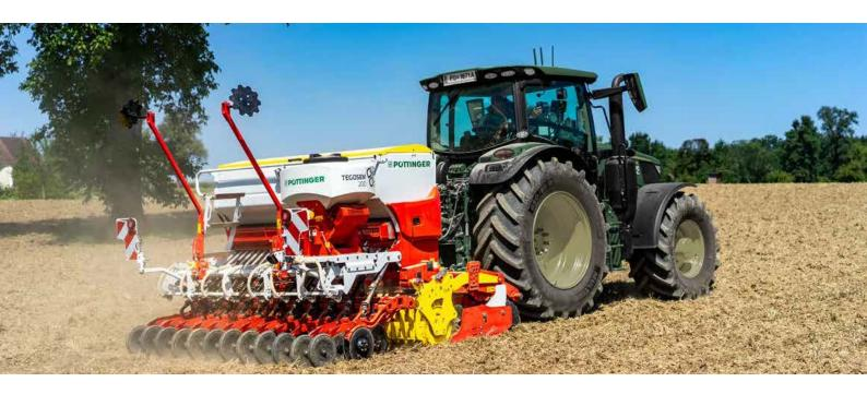
The flexible TEGOSEM hopper combines soil cultivation and sowing a cover crop or a companion crop in a single pass to save time and costs. The TEGOSEM can be combined with both linkage mounted and trailed machines.
