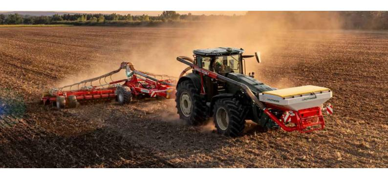
The AMICO F hopper in combination with various arable machines offer the possibility to apply fertiliser or microgranules, cover crops or two components, at the same time. With capacities of 1,700 and 2,400 litres and a division of 60:40, a wide range of applications is guaranteed.
