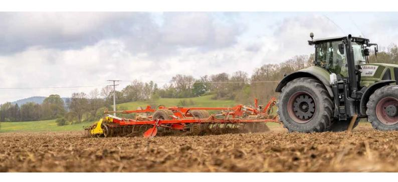
Regardless of whether its stubble cultivation and weed control, incorporating cover crops or seedbed preparation, the trailed PLANO shallow cultivator is the specialist in soil water conservation and mechanical weed control thanks to its shallow, full-surface slicing action. Medium-depth tillage down to 15 cm is also possible for a high output, cost-effective and energy-efficient application.
