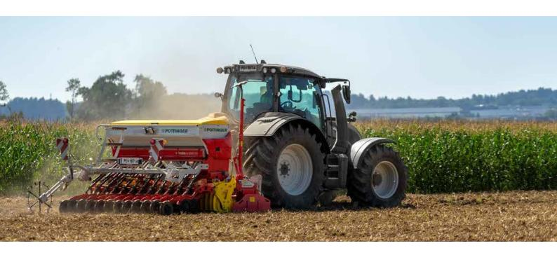
Proven technology meets user-friendly, practical features, all in the latest generation of mechanical VITASEM seed drills. The machines are available as simple linkage-mounted seed drills and with the suffix M (mounted) as implement-mounted machines.
