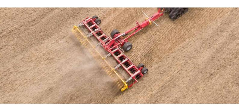
The TERRADISC compact disc harrow is designed specifically for stubble cultivation and seedbed preparation. The compact design and aggressive disc angle ensure reliable penetration and excellent mixing in of harvest residues.
