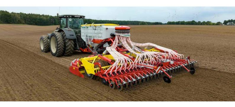
The trailed AEROSEM seed drill combination with active tillage combines seedbed preparation with a LION power harrow, consolidation with a grooved tyre packer and sowing with the DUAL DISC coulter rail. The trailed seed drill concept has been developed for light to the heaviest soil types and enhanced with the profiline comfort control system. This lets you control all the hydraulic functions, including coulter pressure adjustment, conveniently from the tractor cab.
