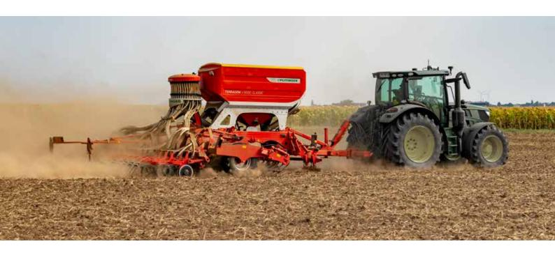
The TERRASEM V CLASSIC models without tillage tools offer smooth running and high output technology for covering large areas. When using these seed drills, the seedbed has already been optimally levelled in advance. Perfect seed placement in a consolidated seedbed is achieved thanks to the optimum ground tracking of the coulter rail and the unique tire packer.
