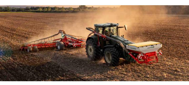
The AMICO F hopper in combination with various arable machines offer the possibility to apply fertilizer or microgranules, cover crops or two components, at the same time. With capacities of 50 and 70 bushels and a division of 60:40, a wide range of applications is guaranteed.
