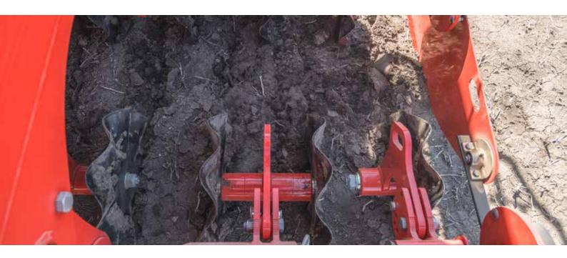
The maintenance-free WAVE DISCs have a diameter of 20" and are available with row spacings of 4" or 6". The working depth is infinitely-variable using a hydraulic system. The PÖTTINGER WAVE DISC system is ideal for difficult soil conditions that require reduced tillage. The WAVE DISC is available for all TERRASEM universal seed drill combinations.
