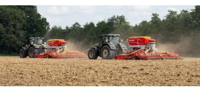
The TERRASEM universal seed drill concept combines tillage, consolidation and drilling in a single machine: the perfect combination of high output, excellent reliability and precision seed placement to meet your requirements. Enhanced by the Profiline comfort control system, all hydraulic functions can be conveniently controlled from the tractor cab.
