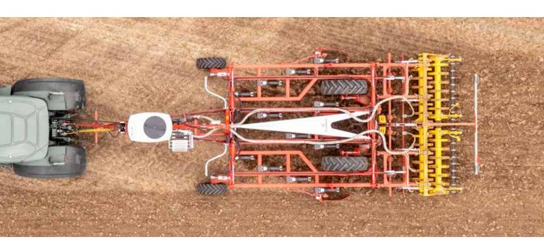
The flexible TEGOSEM hopper combines soil cultivation and sowing a cover crop or a companion crop in a single pass to save time and costs. The TEGOSEM can be combined with both linkage mounted and trailed machines.
