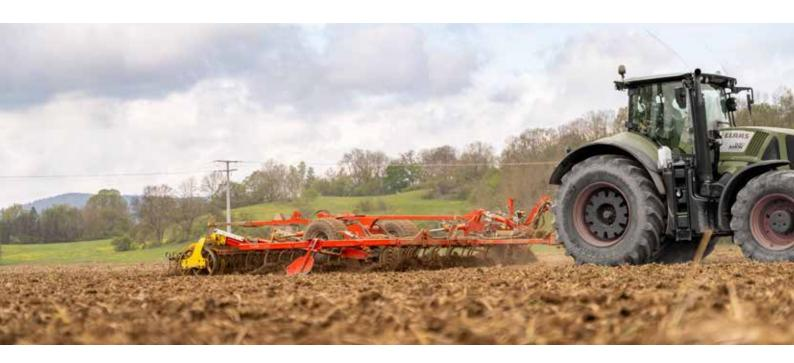
Regardless of whether its stubble cultivation and weed control, incorporating cover crops or seedbed preparation, the trailed PLANO shallow cultivator is the specialist in soil water conservation and mechanical weed control thanks to its shallow, full-surface slicing action. Medium-depth tillage down to 6" is also possible for a high output, cost-effective and energy-efficient application.
