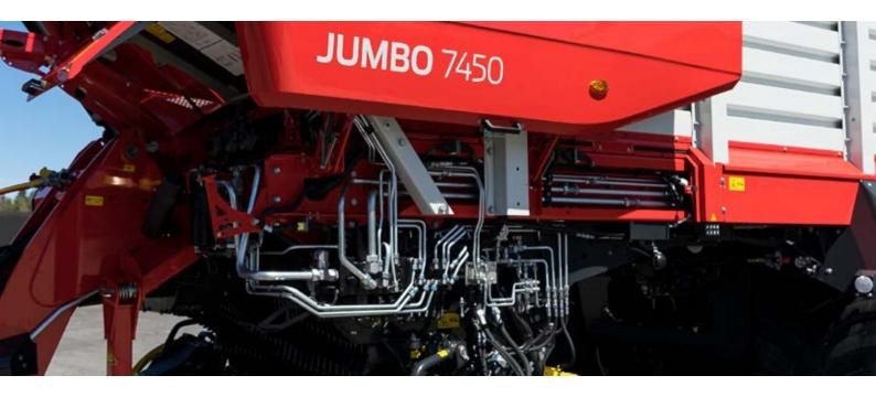
Thanks to the separation of hydraulics and electrics the loader wagon can be cleaned more easily and effectively. The cables are arranged clearly, making it easier to detect faults and reduce downtimes.
