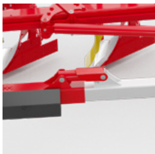
Front furrow width hydraulically adjustable
