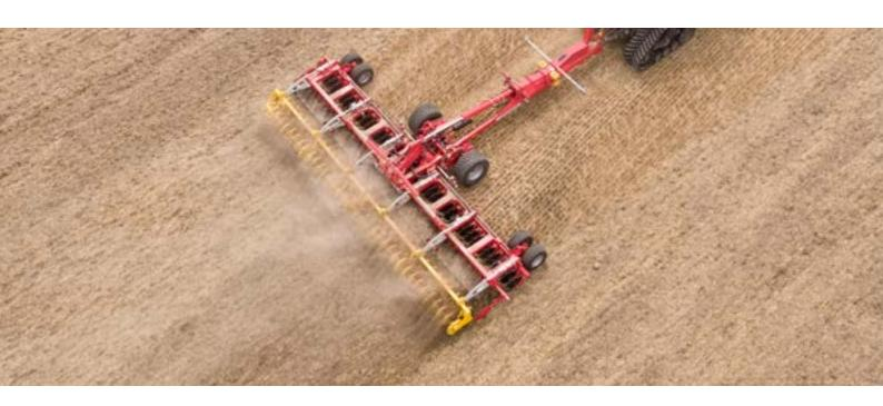
The TERRADISC compact disc harrow is designed specifically for stubble cultivation and seedbed preparation. The compact design and aggressive disc angle ensure reliable penetration and excellent mixing of harvest residues.
