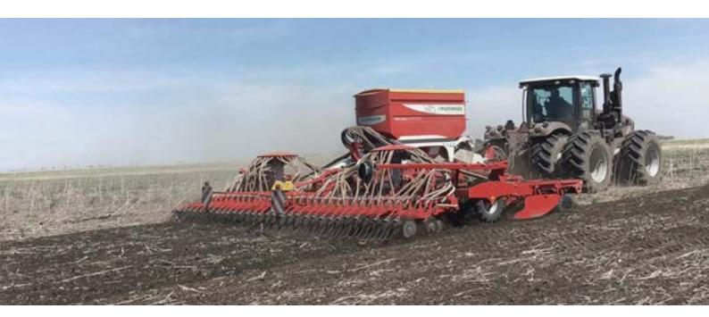
The PÖTTINGER TERRASEM mulch drilling concept combines soil preparation, consolidation and drilling in a single machine. The effective compact disc harrow, unique tyre packer and perfectly designed coulter rail deliver optimum results.
