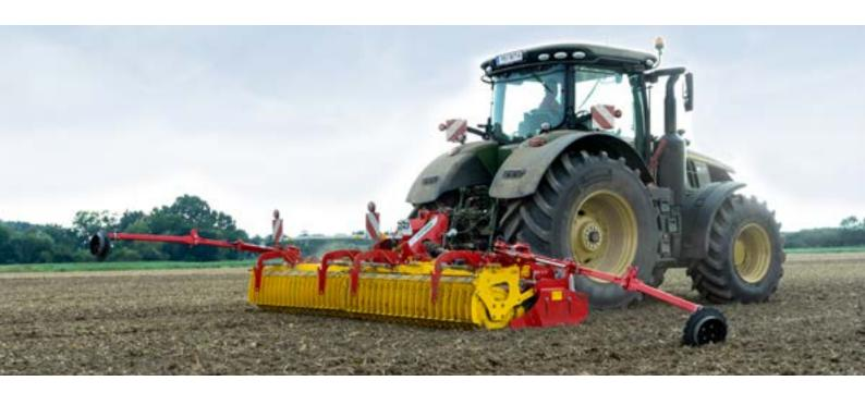
Intensive crumbling for the best quality tilth and excellent mixing of the soil are the highlights of PÖTTINGER power harrows. Combined with a PÖTTINGER seed drill, this machine becomes a high output and cost effective combination that gives you perfect drilling results.
