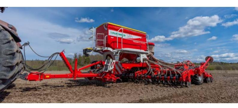
The new TERRASEM CLASSIC models without tillage tools offer smooth running and high output technology for covering large areas. When using these seed drills, the seedbed has already been optimally prepared in advance. Perfect seed placement in a consolidated seedbed is achieved thanks to the optimum ground tracking of the coulter rail and the unique tyre packer.
