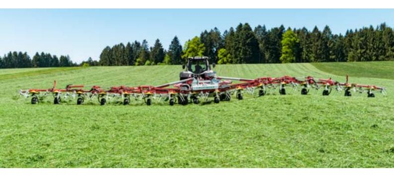
Our proven rotary tedders deliver perfect ground tracking. Both the mounted and trailed tedders feature jockey wheels located close to the tine arc to react to any bumps. In addition, all frame joints follow every contour independently of one another. The tines do not touch the ground. Tedding crops carefully without dirt ingress is the result.
