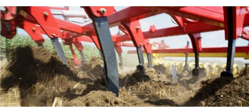
The PÖTTINGER SYNKRO cultivators have been developed to deliver optimum stubble cultivation, and are suitable for both shallow and deep tillage. During the design phase, special value was placed on reducing draft and power requirements.
