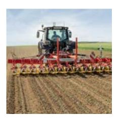
Thanks to its unique design, the new FLEXCARE vario hoe made by PÖTTINGER offers full flexibility working in a variety of crops. The row spacing, the working width of the hoe elements and the fine adjustments of the finger hoe are completely adjustable without the need for tools. The machine features precise depth control and crop-conserving operation. Enclose
